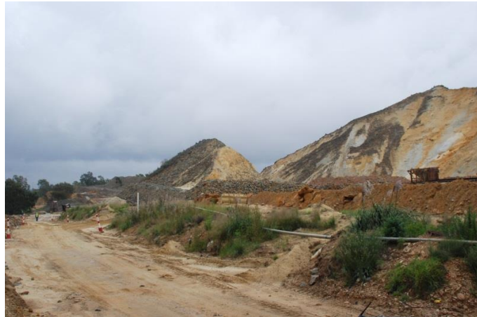
Figure 6: Gold mine tailings re-mining operation of exposed (vegetation removed) tailings dump
